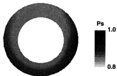
Fig. 24 Exit static pressure distribution produced by 90 deg, one-per-revolution screen on the 100 percent speedline
