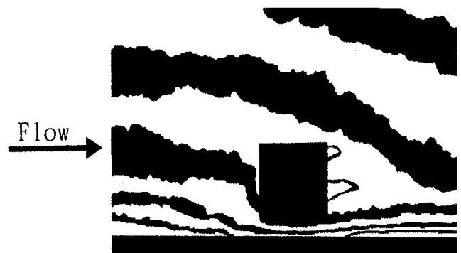
Fig. 8 Example of holographic interferogram for Re = 2 \times 10^4 , C/H = 0.38 , H/De = 0.081 , Pi/H = 10 , and \beta = 44 percent
